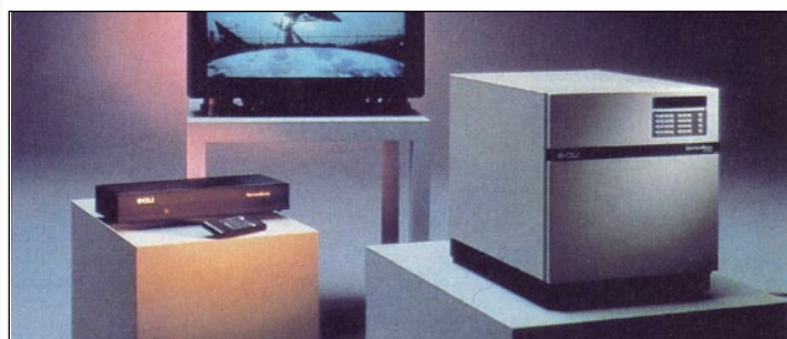
Coder and Decoder of the "Spectrum Saver" by CLI: a regular analogue signal is digitalized to save satellite bandwidth.
